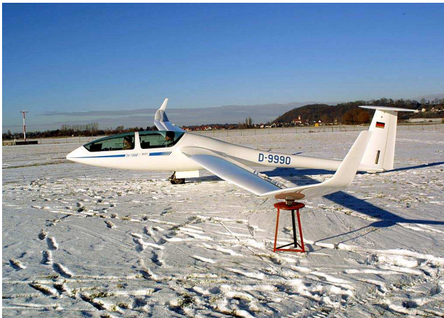
About to start an aertow in the snow -- note footstool used to keep wingtip out of the snow.
